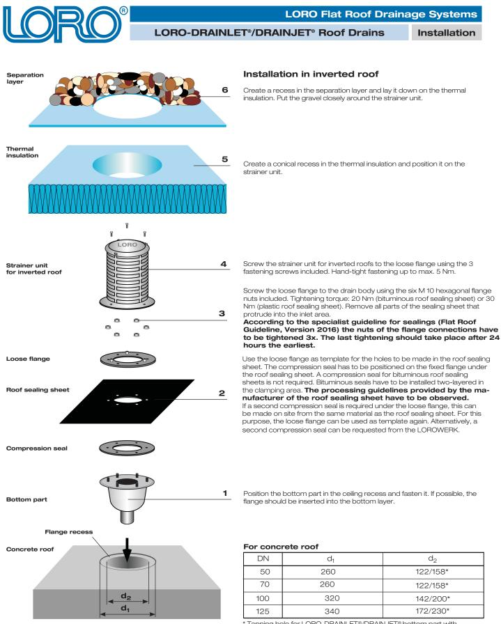
Tapping hole for LORO-DRAINLET®/DRAINJET® bottom part with thermal insulation (two-piece version).
